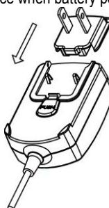
Connect the AC Adapter plug to the input jack.
